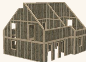
Wood (frame construction)
